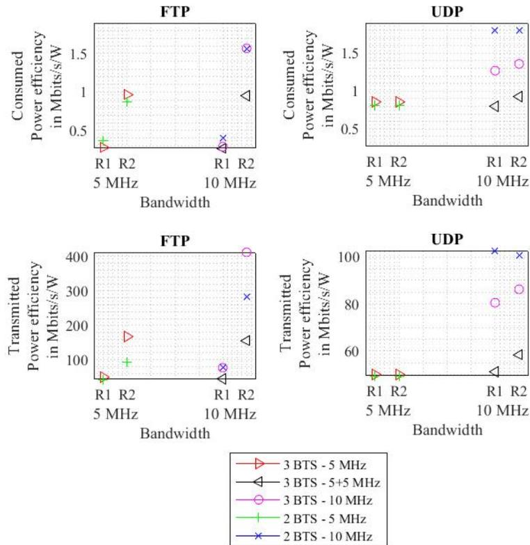
Fig. 8. Variation in the network power efficiency performance between small and large bandwidth usage in the high transmitted power case.
